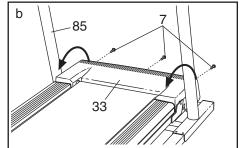
Locate the Reed Switch (22) and the Magnet (18) on the left side of the Pulley (17). Turn the Pulley until the Magnet is aligned with the Reed Switch. **Make sure that the gap between the Magnet and the Reed Switch is about 1/8".** If necessary, move the Reed Switch slightly using a slotted screwdriver. Reattach the Hood (33), making sure that the Screws (7) are inserted into the same holes from which they were removed. Run the treadmill for a few minutes to check for a correct speed reading.
